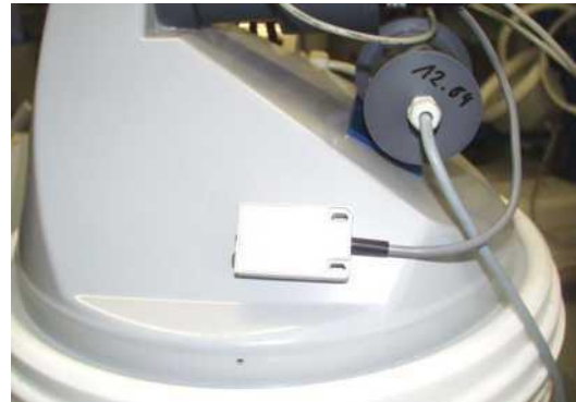
Figure 57, Empty switch mounted on GR 45/100
